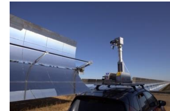
On site receiver inspection system developed by CENER
